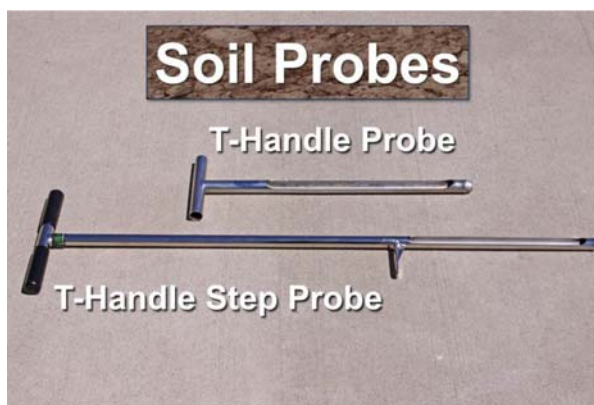
Figure 4: Soil probes provide a simple method for collecting soil samples Photo by Joe Boggs, Ohio State University Extension.
